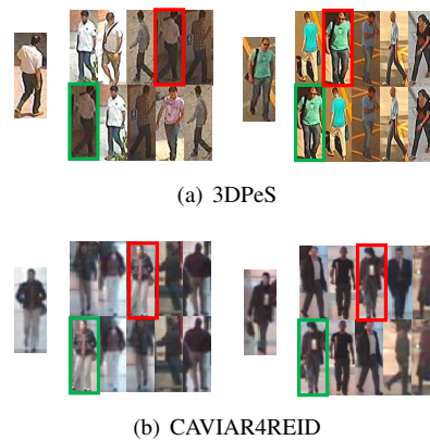
Fig. 12. Top 5 matching gallery images on 3DPeS and CAVIAR4REID. In each group of images, the probe image is on the left. The first and second rows are the matching results of LOMO and LOMO+TED when using MLAPG metric. The bounding boxes show the correct matchings.
