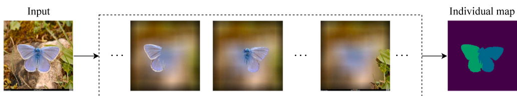
Fig. 3. Demonstration of the pre-segmentation based input partition strategy. The input image is segmented into multiple parts (i.e., super-pixels) using the felzenszwalb segmentation method. Each part together with the smoothed other parts was used as the input, and the corresponding output represents the importance of the image part to the original classifier prediction.
