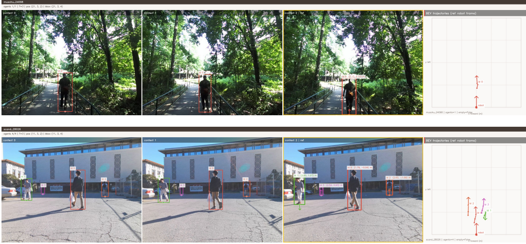
Figure 4: Examples of RGB-based pedestrian localization on MuSoHu (top) and SCAND (bottom). The RGB context frames show the detected pedestrians, their image-space foot points, and the corresponding metric positions. The rightmost panel shows the estimated pedestrian trajectories in the reference robot frame used by the social perception module.
