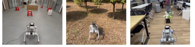
Fig. 3: Evaluation environments. Left: indoor scene with dense static obstacles. Middle: outdoor environment with natural terrain. Right: indoor scenario where an unexpected obstacle is introduced at close range ( \sim 0.5 m) during robot motion to test emergency avoidance capability.
